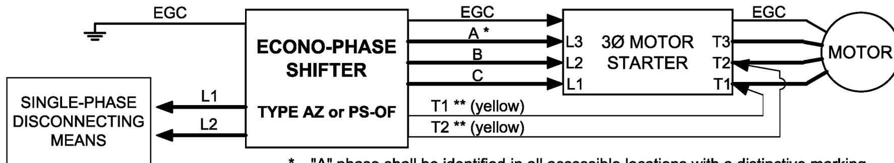
\* "A" phase shall be identified in all accessible locations with a distinctive marking per NEC 455-6 (b). Do not connect control circuits or other single-phase loads to "A" phase (phase with highest voltage to ground when running) from the converter.
